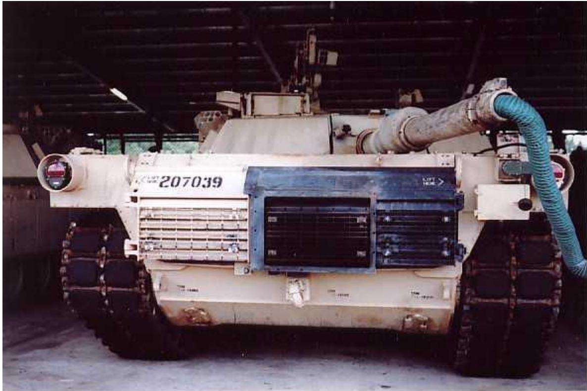
The rear end of the Beast showing a dehumidifier pipe coming from the barrel. This is to stop moisture getting into the computer gear.
