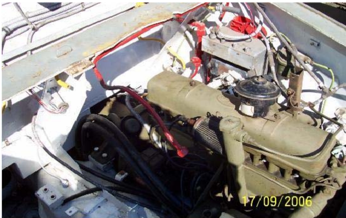
First of the two engines is now in place
